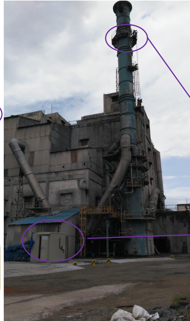
Transmitter and receiver units being installed at the Prill Tower for the measurement of NH 3
