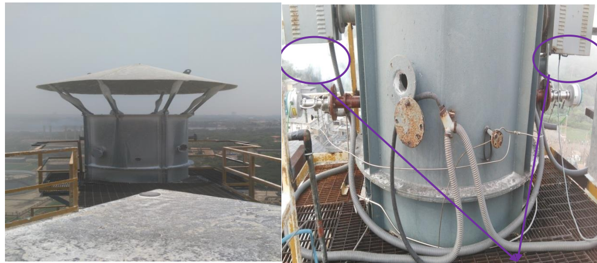
Transmitter and receiver units being installed at the Prill Tower for the measurement of NH 3
