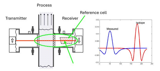
Built-in reference cell with non-interfering gas, here: <sup>18</sup>O<sub>2</sub>
